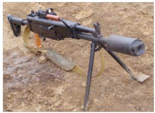
Note the muzzle brake at the end of the suppressor.
