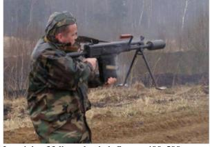
It weights 33 lbs unloaded, fires at 400-500 rpm and is 47" in length. It was never adopted by any armed forces. If such a powerful shoulder fired gun was needed, a much more efficient cartridge would probably be designed.
