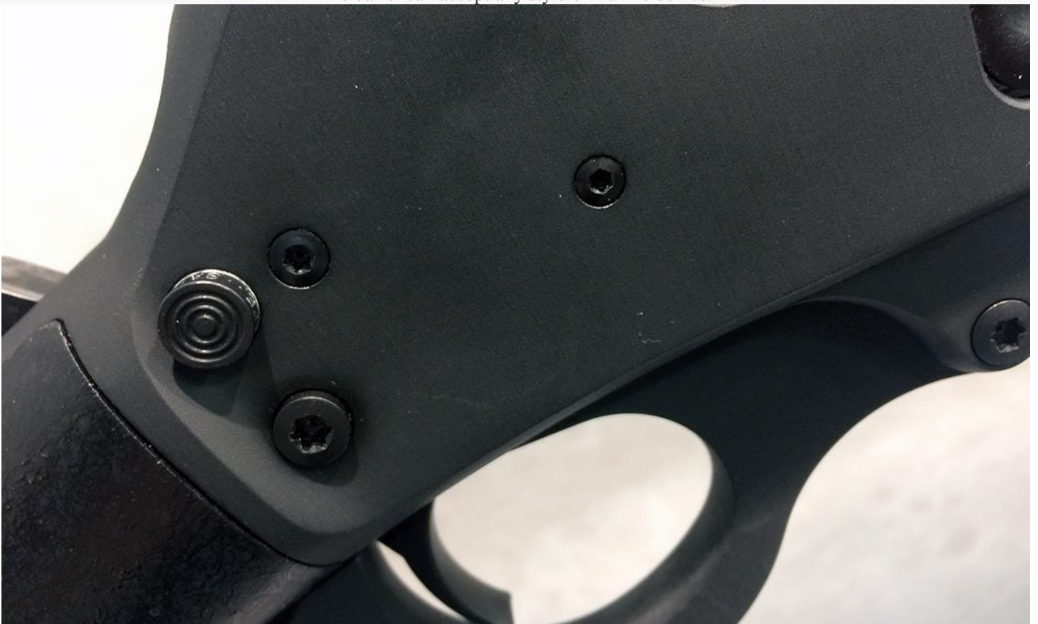
Torx head screws don't strip as easily as flathead screws.
