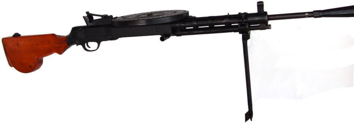
The Soviet DP-28 featured a "pan" magazine not technically a "drum" magazine (Photo: Collection of the Author).
