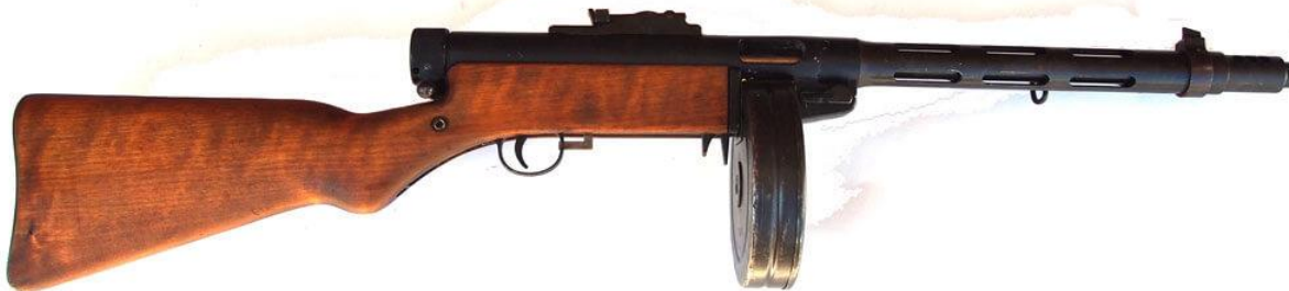
The Finnish Suomi KP/-31 was a reliable and rugged gun, and likely inspired the Soviet-designed PPSH-41. It used the 71-round magazine (Photo: Collection of the Author)
