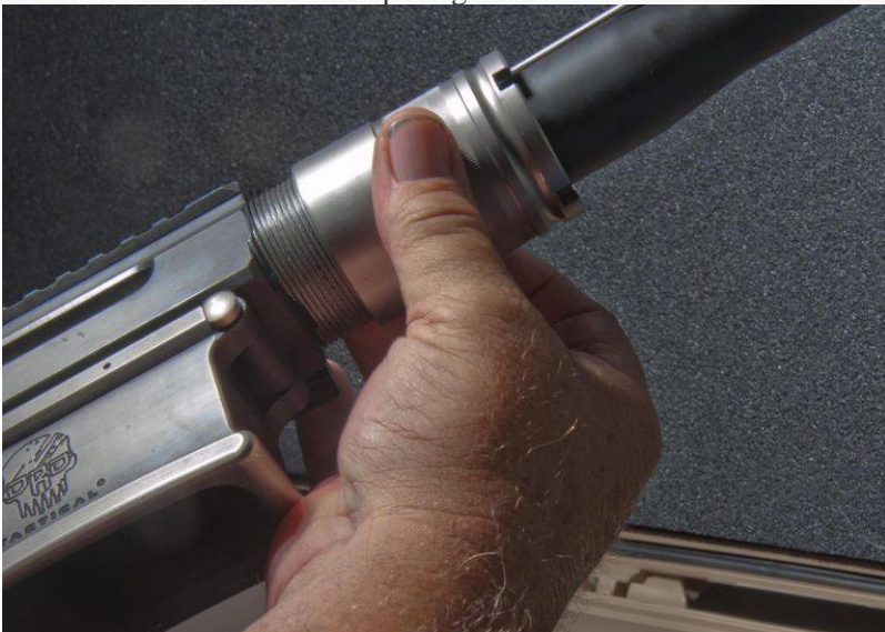
TAKEDOWN STEP 3: Tighten the barrel nut by hand first making sure not to cross thread.
