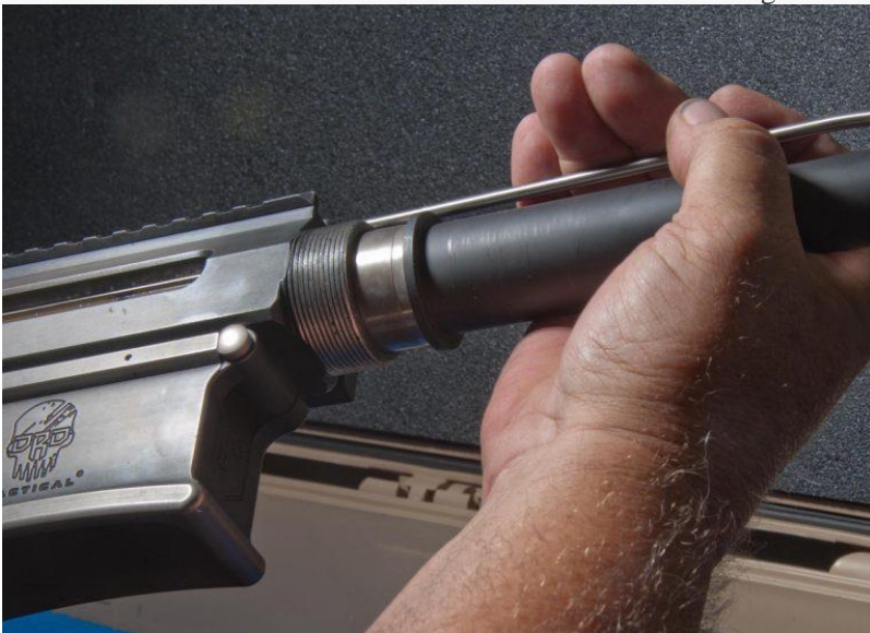
TAKEDOWN STEP 2: Line up the gas tube and the barrel and then lock into place.
