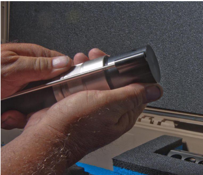
TAKEDOWN STEP 1: Loosen the barrel nut and remove the gas tube and chamber protector.
