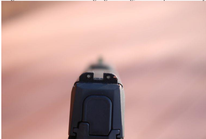
The rear sights have a shelf for one-handed manipulation, should the need arise.
