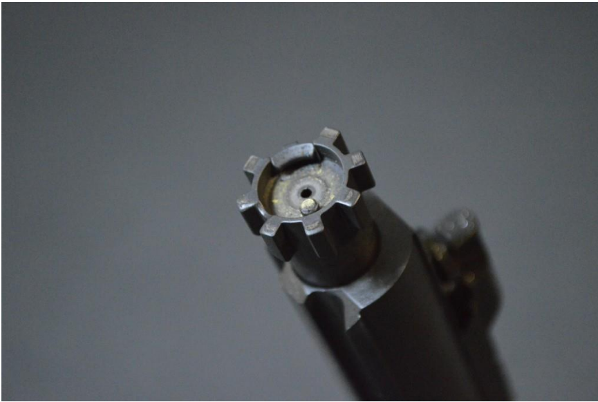
A look at the MkG Banshee's .45 ACP bolt head. The 9mm version's is essentially the same.
