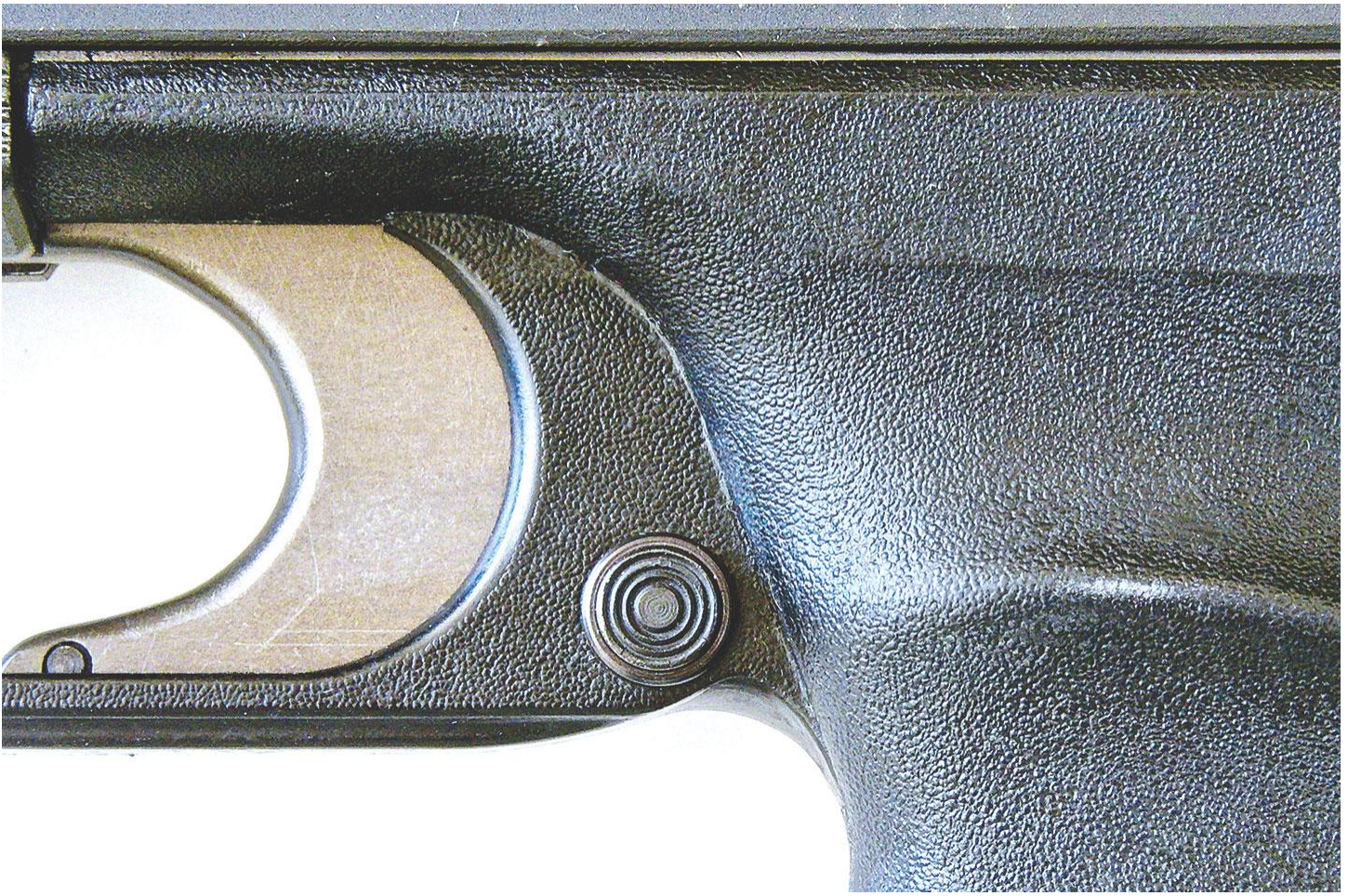
Close-up of the VP70's cross bolt safety.
