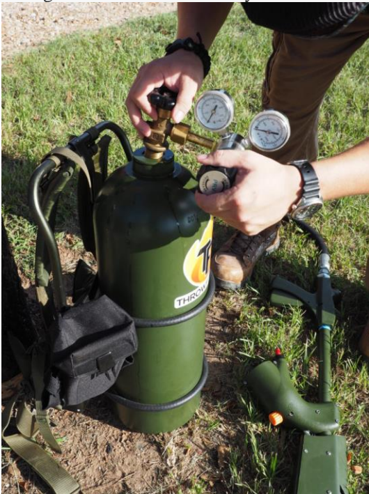
Finally screwing on the regulators so we can pressurize the tank.
