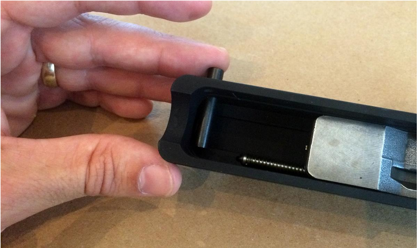
Step 2: Install the Bolt Stop Pin This one is pretty self-explanatory.
