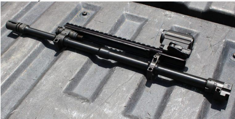
The barrel, with rail attached. This method of mounting the rail gives more stability than you would get from mounting the rail to the polymer parts.
