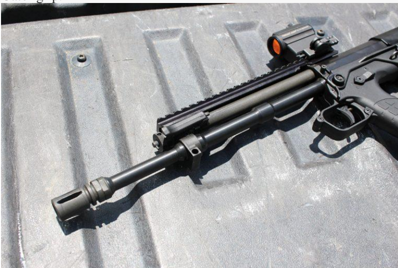
The gas tube sits about where it would on a carbine length AR, but this system is adjustable.
