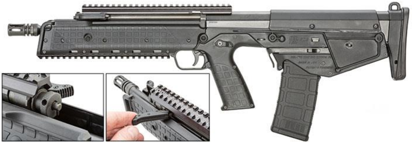
The downward-ejecting RDB (above), shown with a 30-round PMAG, employs a forward-mounted charging handle (inset, r.) that is switchable for left- or right-hand use. The rifle's gas system is adjustable (inset, l.) without tools and comes factory set for M193 55-gr. 5.56x45 mm NATO ammunition.
