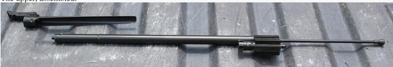
The bolt carrier contains the recoil spring—the thin plunger sticking out the back end.
