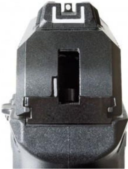
The drift-adjustable U-shaped rear and white-dot front sights sit within large dovetails.
