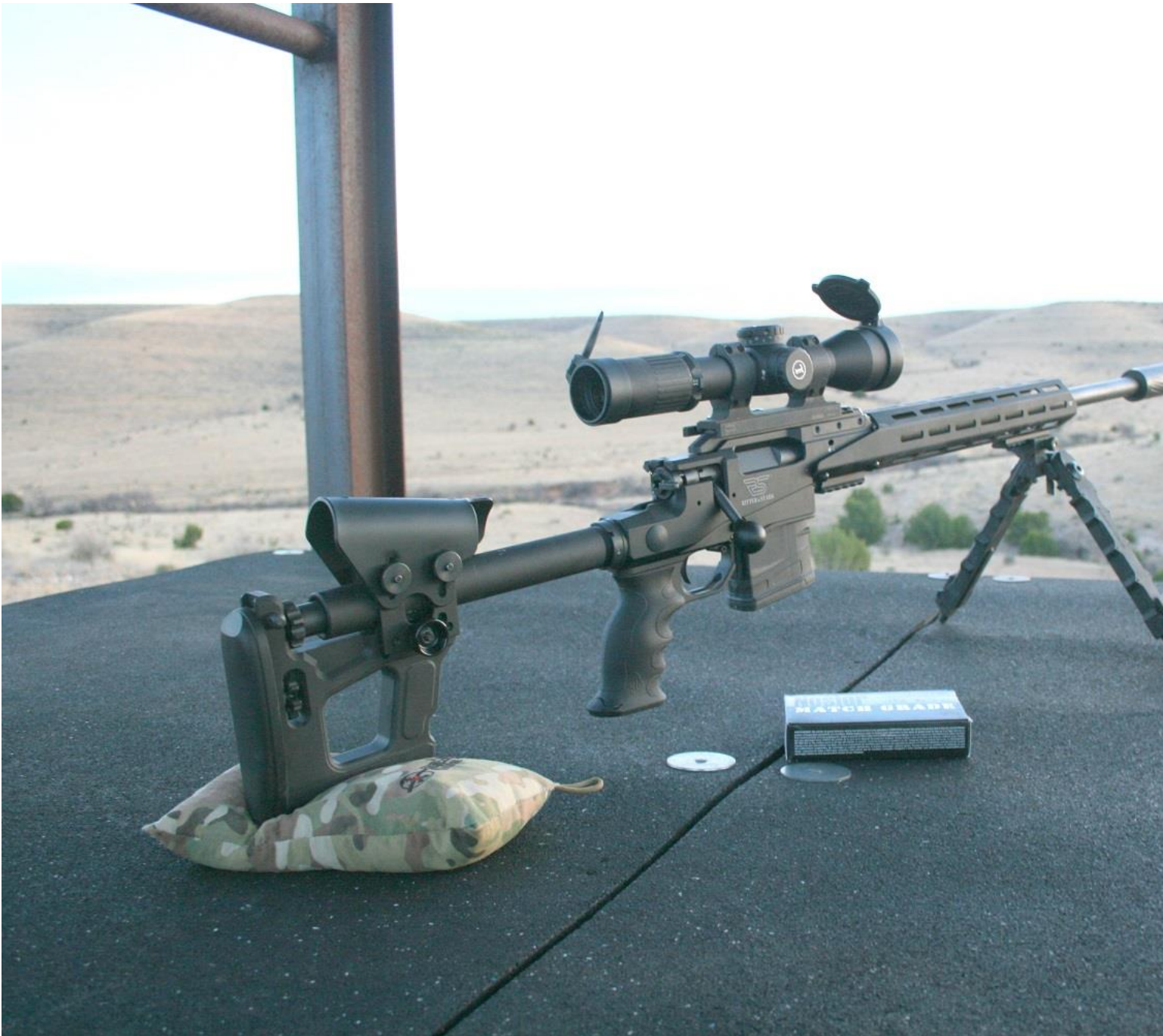
Ritter and Stark SLX chambered in .308 Winchester. The tough-as-nails Accu-Tac SR-5 bipod and the Thunder Beast arms suppressor made this rifle a joy to shoot. Note the comb on this rifle. I configured it so it sloped towards the receiver. When the rifle recoils to the rear, the shooter's face stays in-line with the rifle scope.
