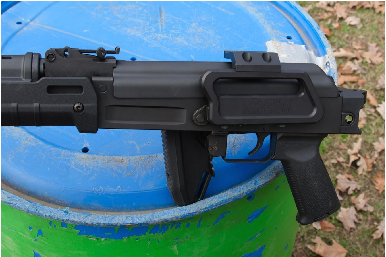
The Zhukov-S stock folds along the right side of the receiver and does not interfere with the scope mount.
