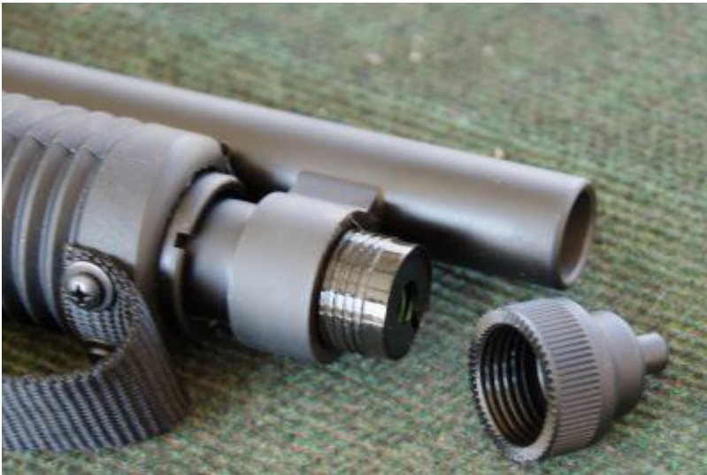
The tubular magazine is capped off with a threaded and removable end cap.
