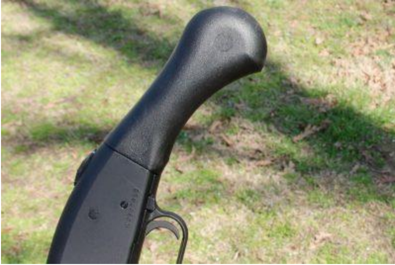
The Raptor grip is curved and proved to help dampen the recoil of the 12 ga.
