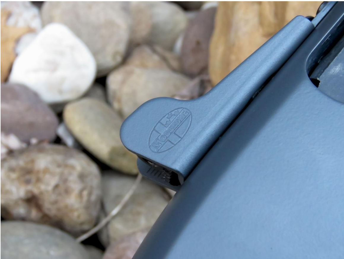
By applying coats lightly so they build up a little each time allows small details like this Mossberg logo to show up.
