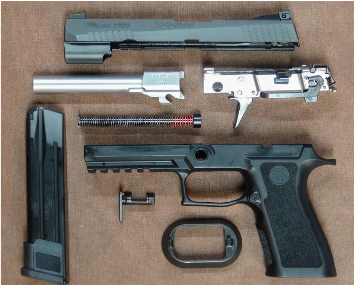
In addition to the usual P320 components, the X-Five sports a bull barrel, flat trigger, and speed magwell.
