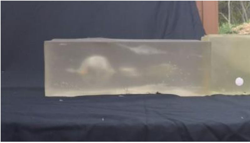
Winchester 223 temporary wound cavity flame beginning to form at rear of temporary cavity.
