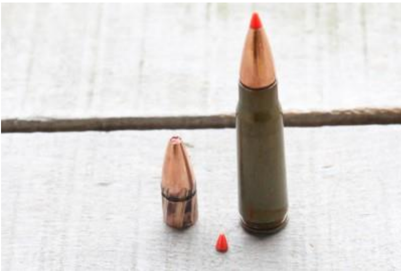
7.62 x 39 bullet retrieved from gel zero expansion ballistic tip broken
