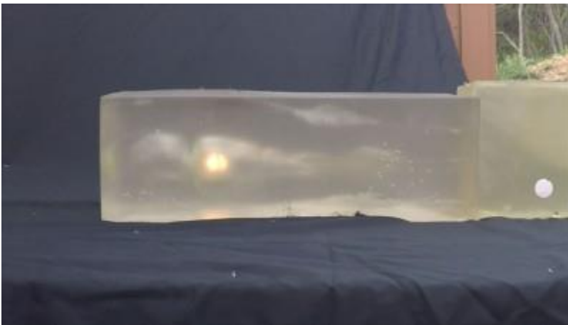
Flame from Winchester 223 caused by burning gases and pressure change from block collapsing on temporary cavity.
