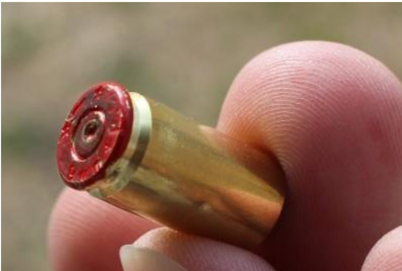
9mm over-pressure test round. Do not reload.
