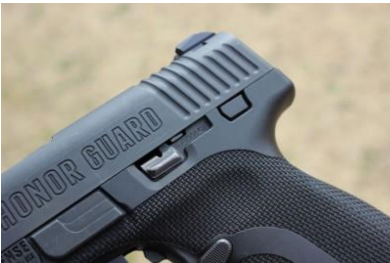
That odd cut-out is where a safety lever would go. That is a plug of sorts.
