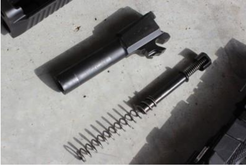
One captured spring inside the more traditional recoil spring.
